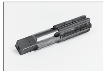
Fig. R88 — ISO 6149-1 Straight Thread Port Tap
