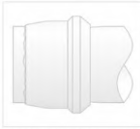
Fig. T47 — Tube not bottomed
