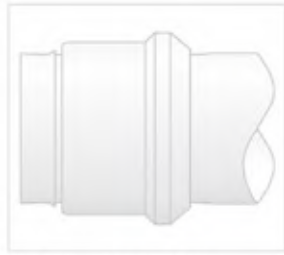
Fig. T48 — Shallow bite
