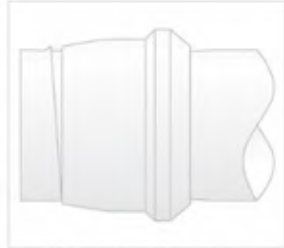
Fig. T50 — Ferrule cocked on tube
