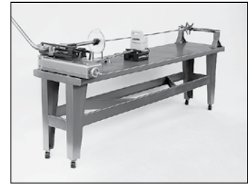
Fig. R31 — Bender Table (equipment not included)
