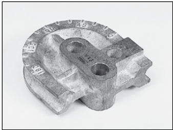
Fig. R27 — Radius Block for use with HB632 Bender
