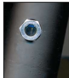
This sight gauge shows the color of the silica gel. When the gel turns from blue to pink, it is time to change the desiccant.
