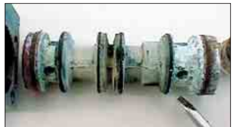
Contaminants corrode and damage air-operated equipment
